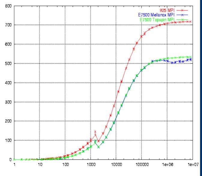
Unidirectional bandwidth (MB/sec) vs message size (bytes) measured with MPI version of Netpipe – PCI-X on E7500
