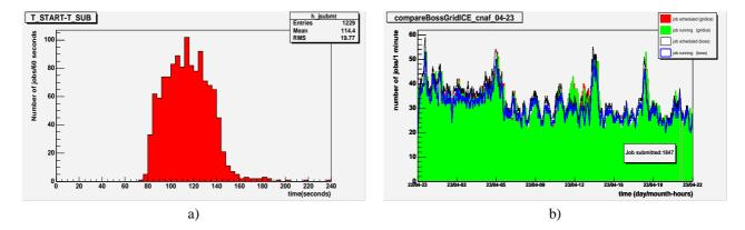
Figure 2: a) Time delay introduced by the grid measured as the difference between the job submission time and the time of start execution. b) BOSS and GridICE distributions of the number of scheduled and running jobs on the 23rd of April at CNAF.
