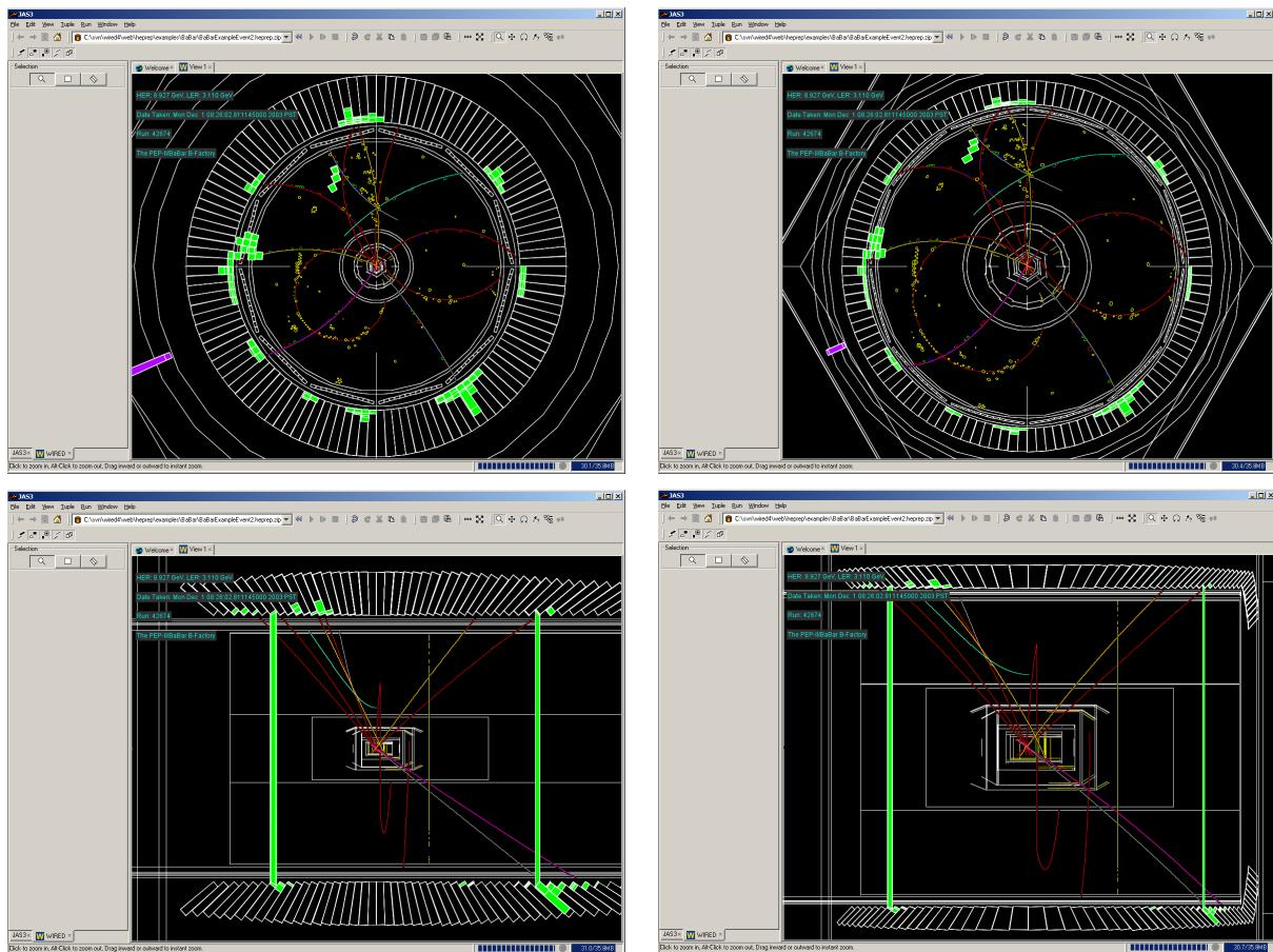
Figure 2: The BaBar detector and an event shown in a XY projection (top-left), shown in a fish eye projection (top-right), shown in a  $\rho$ - $Z$  projection (bottom-left) and shown in a composite projection combining a fish-eye and a  $\rho$ - $Z$  projection (bottom-right).
