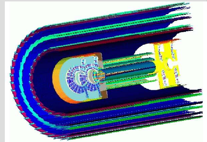
Sliced view of CMS barrel
