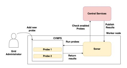
Extensible - Can add or remove new probes to collect metrics without any code changes
