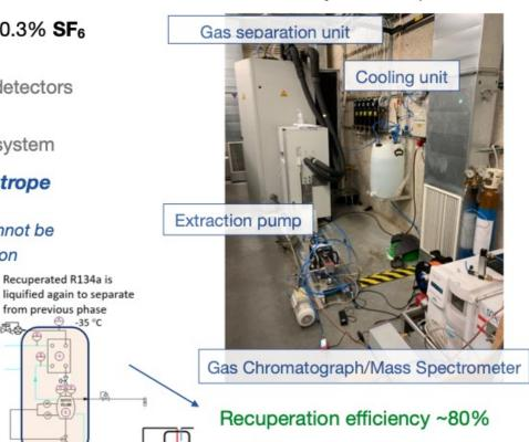
First C<sub>2</sub>H<sub>2</sub>F<sub>4</sub> recuperation system under construction: installation foreseen beginning of 2023 in CMS experiment
