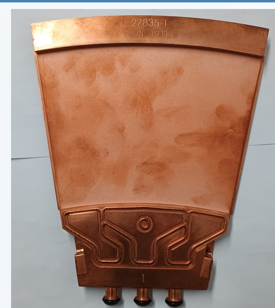
Figure 4: One of 16 micro-channel water-cooled copper petals on to which lithium is directly bonded for neutron production [7,8]. The total heat removed is approximately 100 kW, caused by incident protons stopping within the lithium layer.
