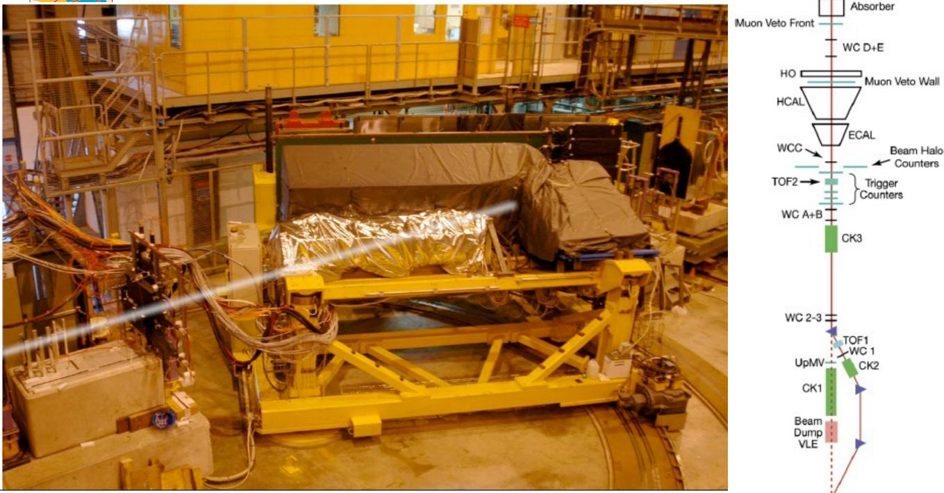
This test beam setup provided measurements of energy response and energy resolution for pi-plus, kaons of either charge, antiprotons of momenta between 2 and 9 GeV, pi-minus of momenta between 2 and 300 GeV and protons of momenta between 2 and 350 GeV
