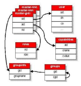
Figure 2: The VOMS database structure
