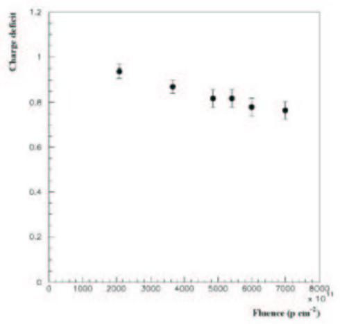
Signal (106Ru B—source) degradation as a function of fluence in a non-homogeneous irradiated detector (n-in-n). Data G. Casse
