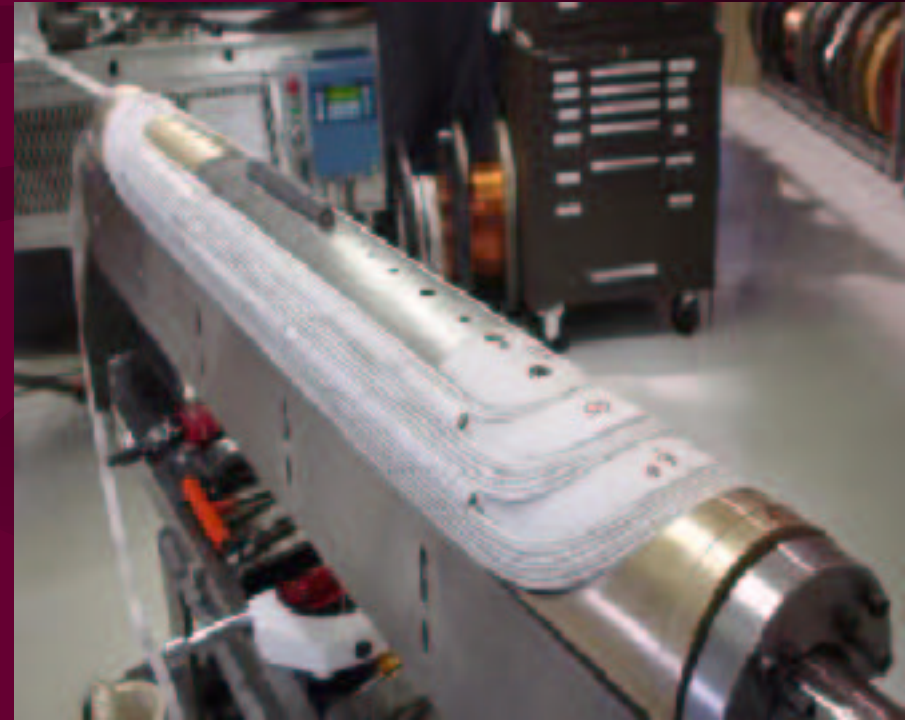
Coils for a mechanical model of a cosine \theta magnet at FNAL. The Nb 3 Sn cable is insulated in ceramic cloth (left).
