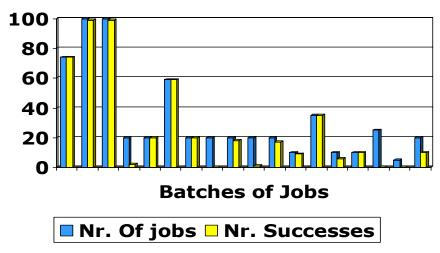
Efficiency was generally a step function for batches (close to 0 or close to 100). With long jobs and multi files very sensitive to long-term system stability
