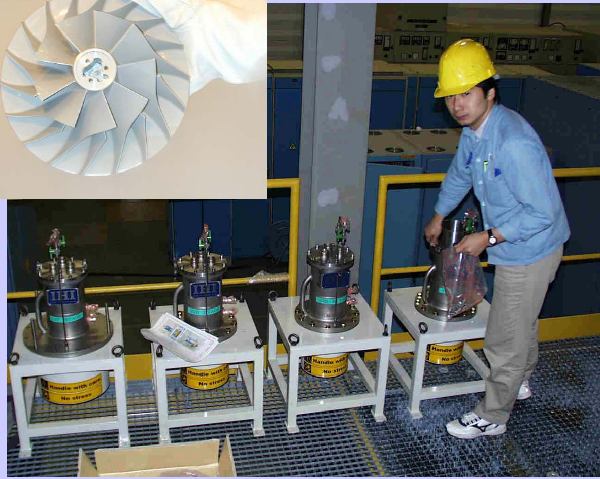
The four-stage LHC cold compressors
