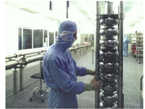
Cleanroom handling of niobium cavities
