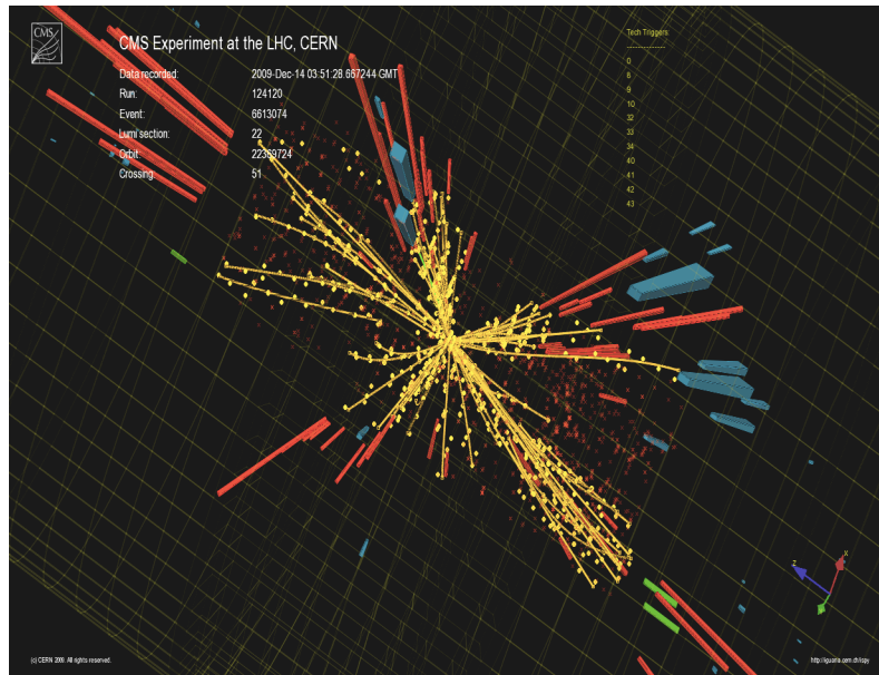
Figure 4: An event display of a “hard” proton-proton collision in CMS illustrating the inner tracking detector hits (yellow) and the energy deposits in the electromagnetic calorimeter (red) and the hadron calorimeter (blue). The height of the red and blue towers is indicative of the energy deposited. The muon system is not displayed. The production of “jets” is evident from the collimated bunches of particles.
