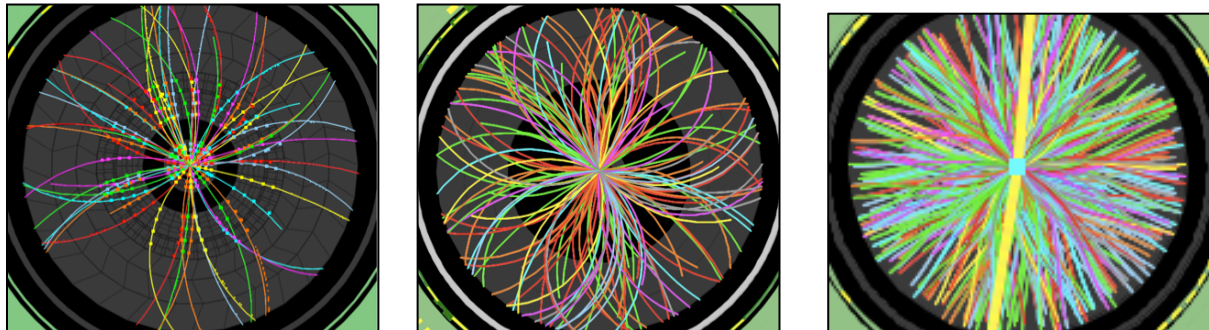
Figure 7: Displays of events recorded by ATLAS in 2010 (left panel), 2011 (middle panel) and 2012 (right panel). Trajectories of charged particles with p_T > 0.4 GeV are shown in transverse views of the tracking detectors. The yellow tracks in the right panel indicate the two muons produced from a Z \rightarrow \mu\mu decay.
