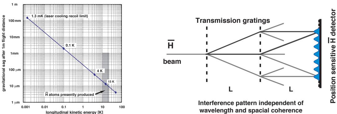
Figure 1: Gravitational sag of  $\bar{H}$  in the earth field after 1 m flight distance (assuming  $\bar{g} = 9.81 \text{ m/s}^2$ ) and a possible interferometer with two identical transmission gratings and the position sensitive  $\bar{H}$  detector.
