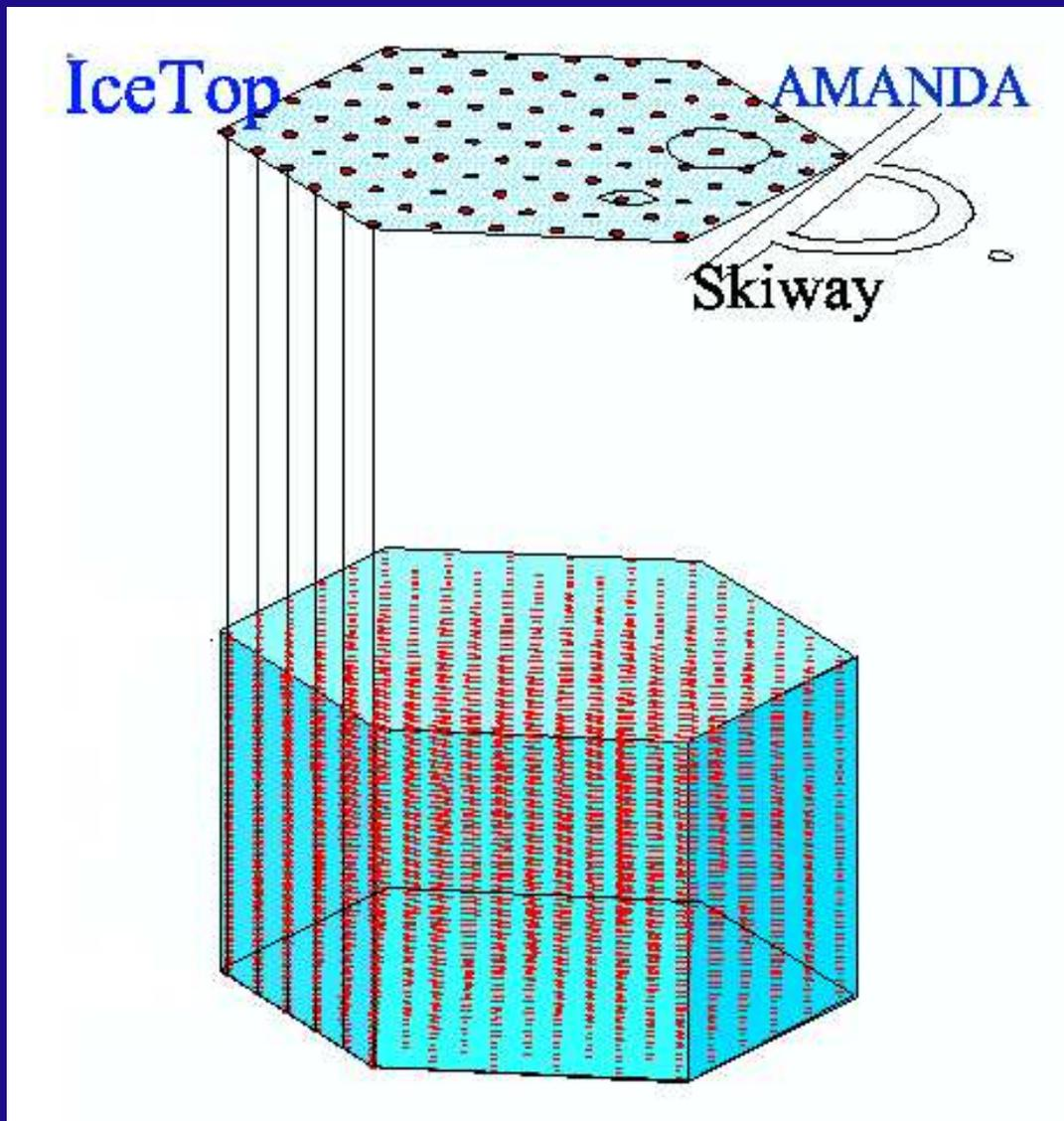
IceCube: 4800 PMTs/80 strings, 60 PMT/string spaced by 17 m. Each string from 1400m to 2400m. Instrumented volume  $1 \text{ km}^3$ . Construction will start austral summer 2004/2005. 16 strings/season.
