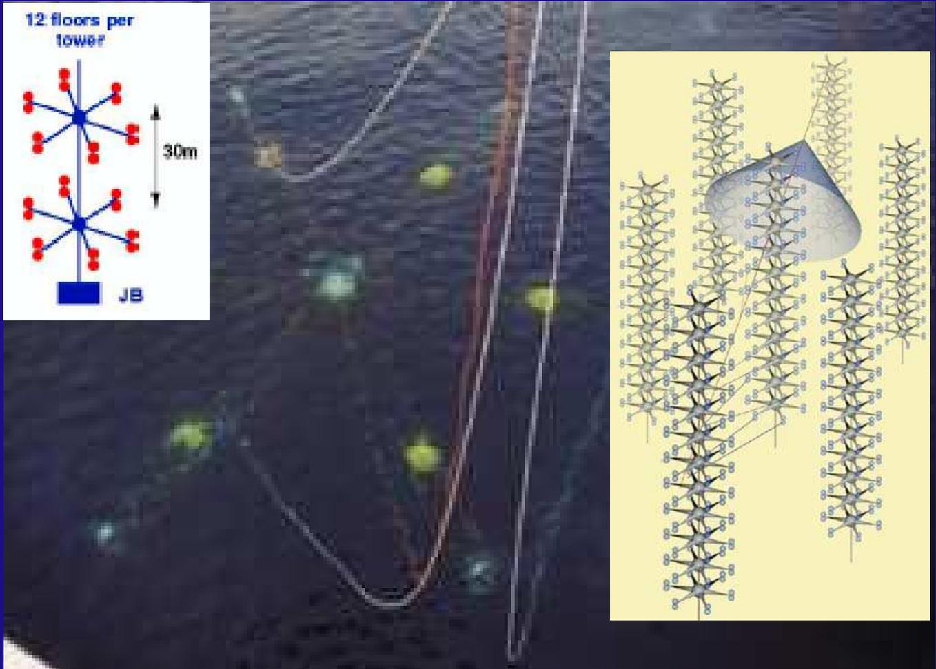
Tower based detector with 12 hexagonal floors spaced by 30m with 6 pairs of up-down looking 15' PMTs each. 4 km depth. Near Pylos (Greece).  $A_{tower} > 0.02 \text{ km}^2$  for  $E_{\mu} > 10 \text{ TeV}$ . 28km electro-optical cable put in 2000 and repaired in 2002.
