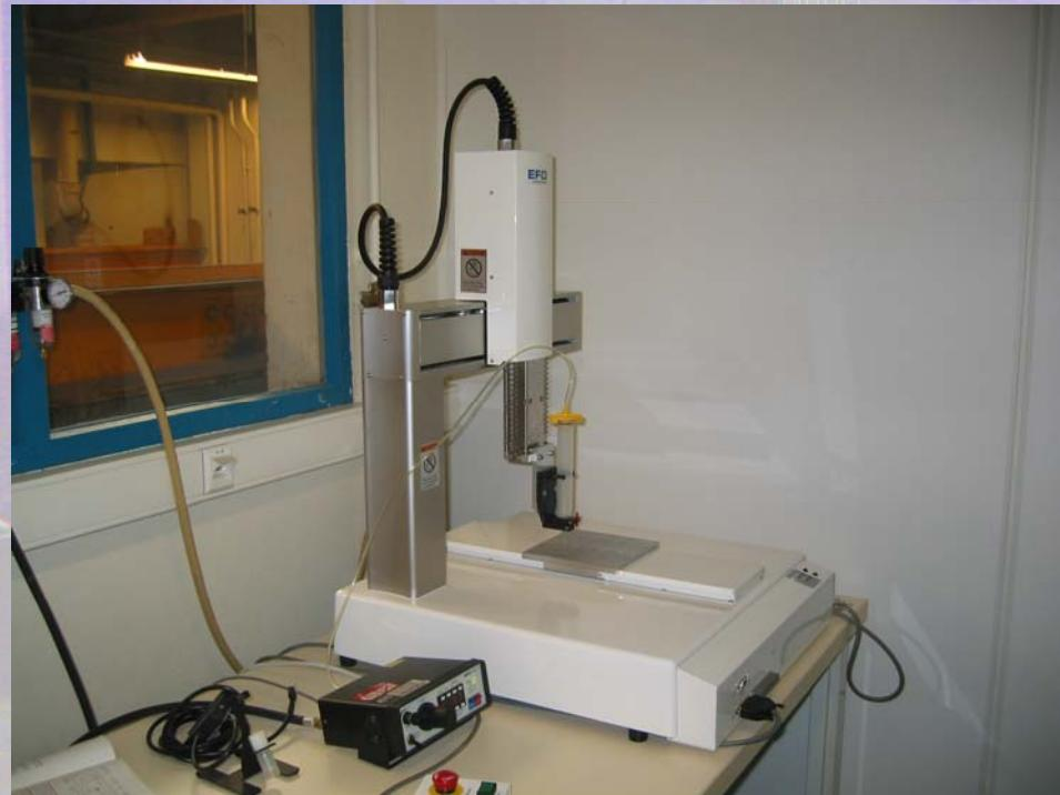
X-Y-Z table ( $400 \times 400 \times 150 \text{ mm}^3$ ) with glue dispensing tool (conductive glue)
