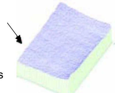
MRF 2micron removal uncovers subsurface scratches
