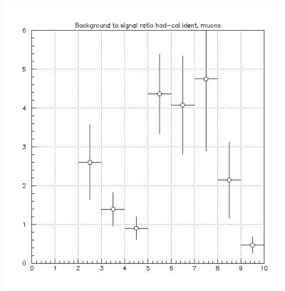
Here one can see where the real problem sets in using (only) the had-cal: the background to signal ratio is very poor, so that what is classified as muon from the calorimetric system has a very high probability of being a hadron instead...
