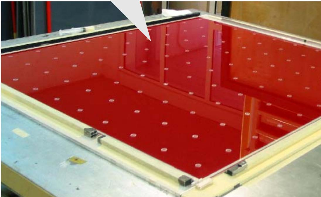
Resistive acrylic paint for electrical contacts deposited with silk screen printing technique
