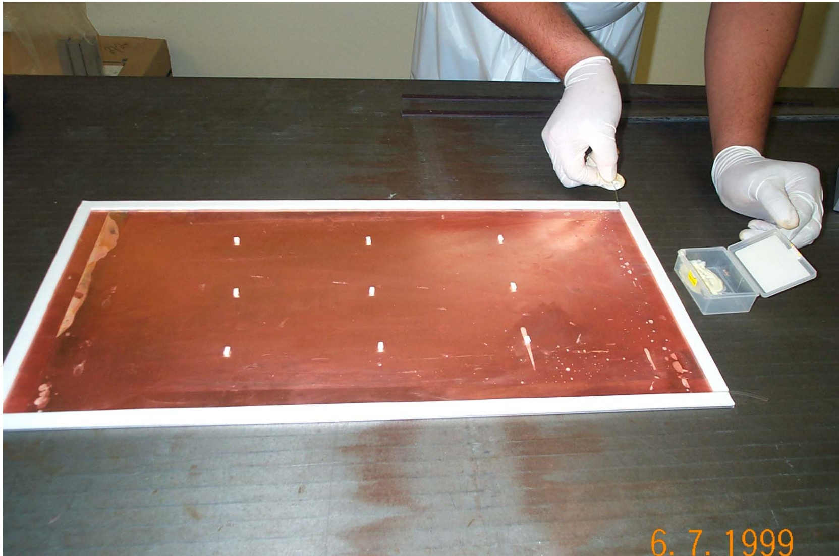
3mm side walls and spacers installed
