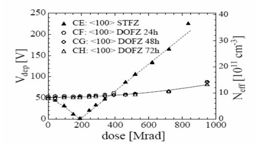
Most remarkable fact: oxygenated Si is impervious to electromagnetic radiation damage, i.e., OK for LC, and not OK for p's and  $\pi$ 's, i.e., not OK for LHC.
