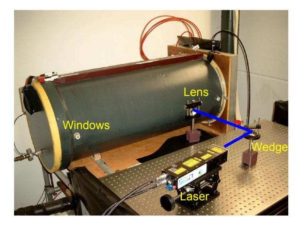
Setup used to produce first laser tracks in the TPC
