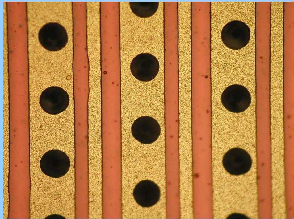
Idea: Negative strip voltage  $\Rightarrow$  Ions are collected on the strips, while electrons, due to diffusion, pass.
