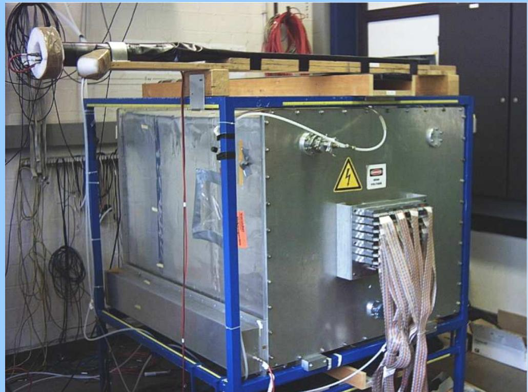
Application of a radioactive  $^{55}\text{Fe}$  source at the cathode exactly opposite of the readout
