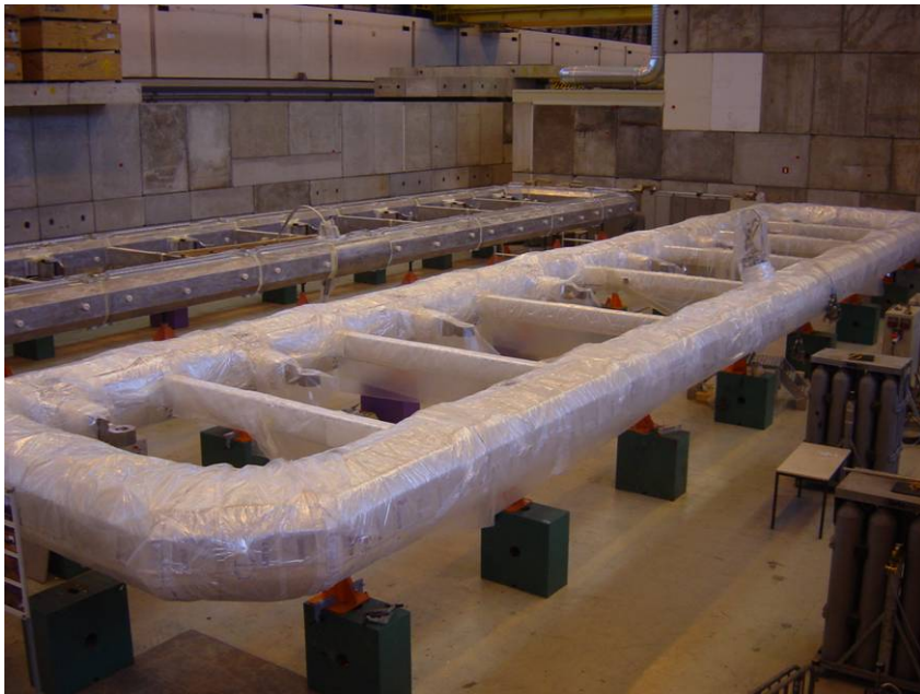
A coil wrapped completely with MLI
