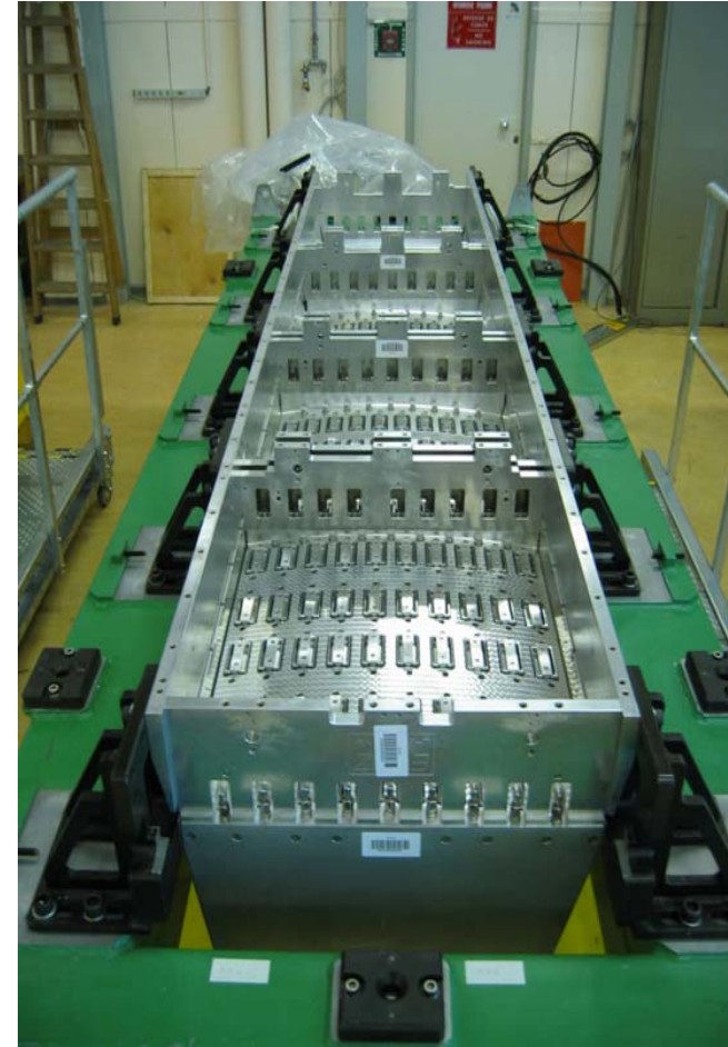
Barrel supermodule (1700 crystals)
