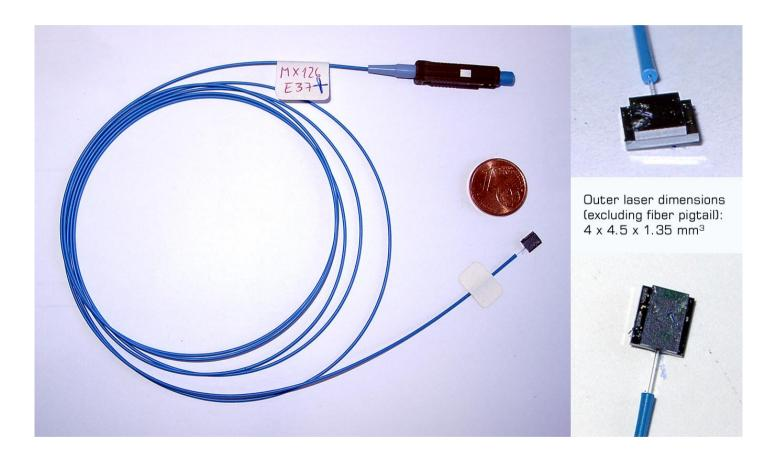
TypePigtailed single-laser pill (no suitable COTS arrays available)ConnectionsElectrical: wire-bonding; Optical: MU connector
