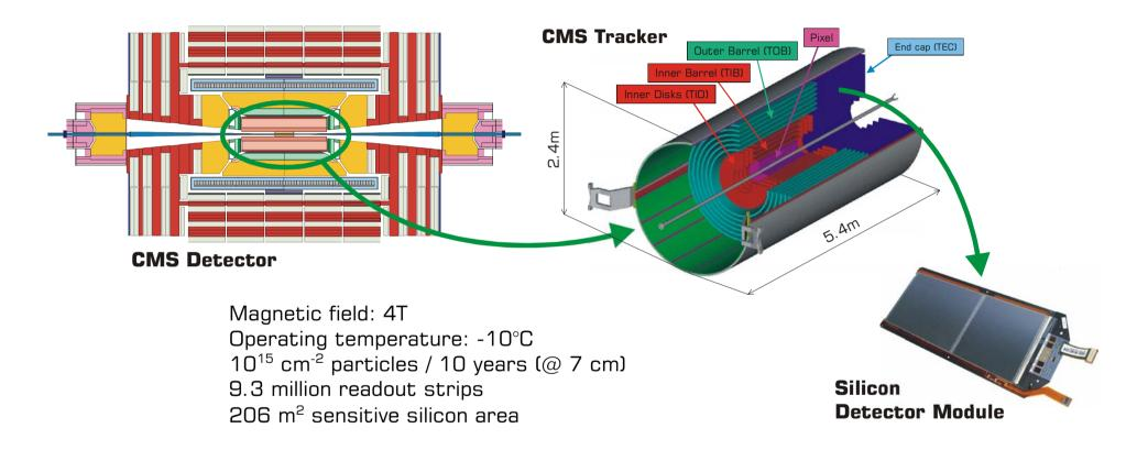
ReadoutAnalog optical readout @ 40MS/s (time-multiplexed strip data)36k optical fibers, 60...100m long
