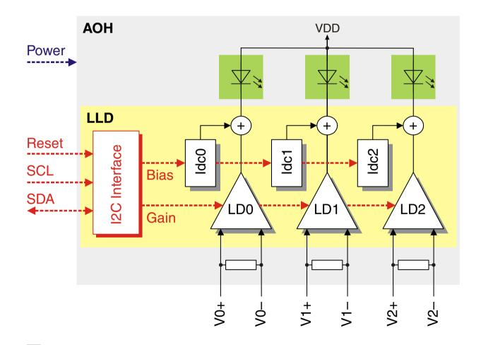
Contents Linear Laser Driver (LLD) and 2 or 3 laser diodes
