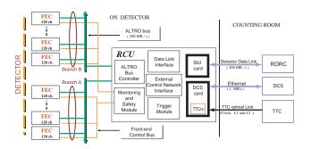
Figure 1: The architecture or the TPC readout electronics. Up to 25 FECs are interfaced via 2 separate branches of the ALTRO readout bus and the local Slow Control link, while other 2 optical links and an Ethernet connection interface the RCU respectively to the Read Out Receiver Card, the Trigger Timing Circuit and the Detector Control System.
