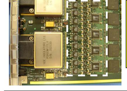
High density components. Close up of analogue sect on primary side (indicated region is repeated on secondary side).
