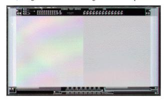
Figure 11. The LCFI/E2V CPC-1 column-parallel-readout CCD prototype.
