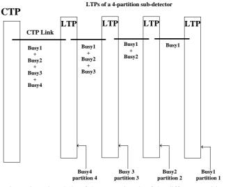
Figure 3: Daisy chain of the Busy signals of the different partitions of a sub-detector
