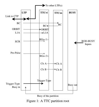
The interface to the CTP is done through a differential link (CTP Link). As the number of TTC partitions in ATLAS is high (a bit less than 40), it is not affordable to have as many CTP Links. Only 20 links will be available, one link per sub-detector. Each CTP Link connects the CTP to all the LTPs of a given sub-detector (and only to these LTPs) using the daisy chain.
