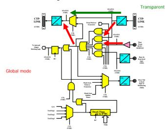
Figure 8: Block diagram of the BUSY path
