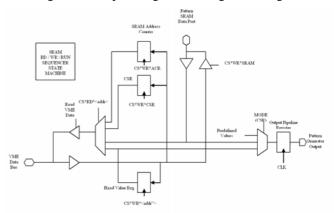
Figure 6: Block diagram of the pattern generator
