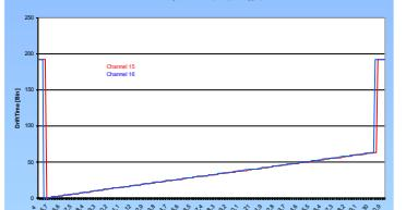
Figure 6: Delay scan (Drift Time vs. Hit Position) of the OTIS 1.1 for 1BX *Encoded Hitmask* mode.
