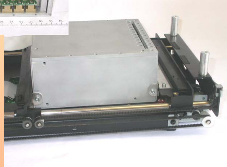
Detection unit of scanner in cover with X positioning motion system up to 14 cm (in 564 (250 \mu\text{m} ) or 1650 (85 \mu\text{m} ) steps)
