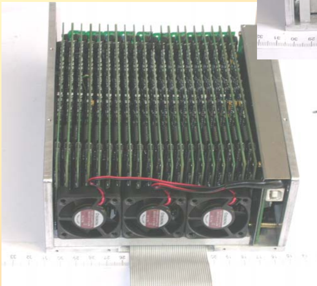
View of opened analog scanner part with cooling system (in front)
