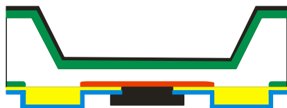
Cross section of a thinned silicon detector
