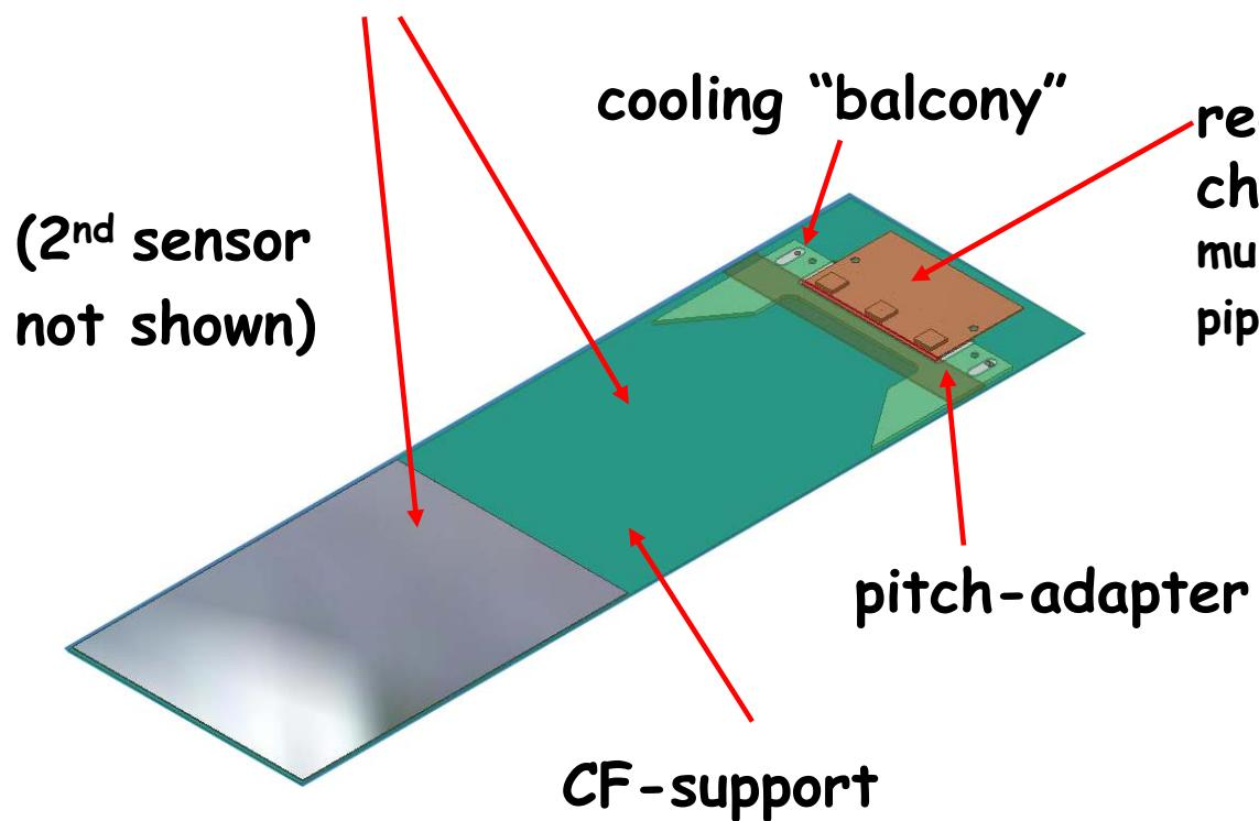
readout hybrid with 3 Beetle chips (40MHz, 128channels, multiplexed on 4 readout ports, pipelined 183BX, 0.25 $\mu\text{m}$  CMOS)
