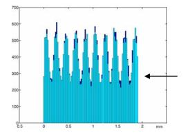
Typical interference pattern (simulation with two gratings 200µm grid spacing 1m apart, 15K atoms, isotrope emission) 100000 atoms emitted ~25000 detected
