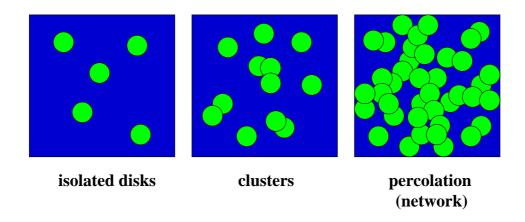
for N disks, disk density n = N/F average cluster size S(n) increases with increasing density n
