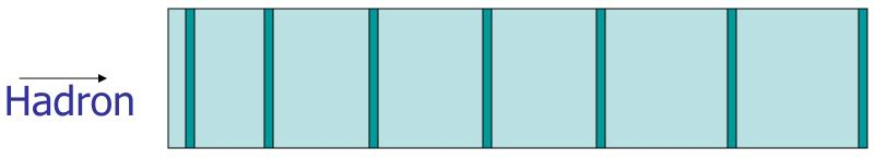
The green is solid metal. Detectors that sample the shower are shown in blue. Detector near front end is for EM shower
