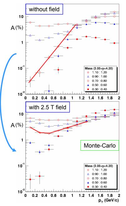
The acceptances depend on the magnetic fields (in the muon spectrometer and in the vertex telescope), on the "thickness" of the muon filter, on the relative distances between the target, the detecting elements and the magnet, etc. They are evaluated through Monte Carlo simulation.
