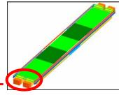
➤ The fiducial marks will be likely to be put somewhere here, on the most external part of the supermodule.
