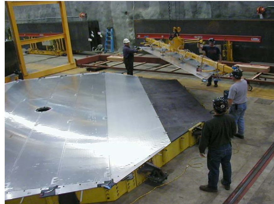
Far Detector plane under construction
