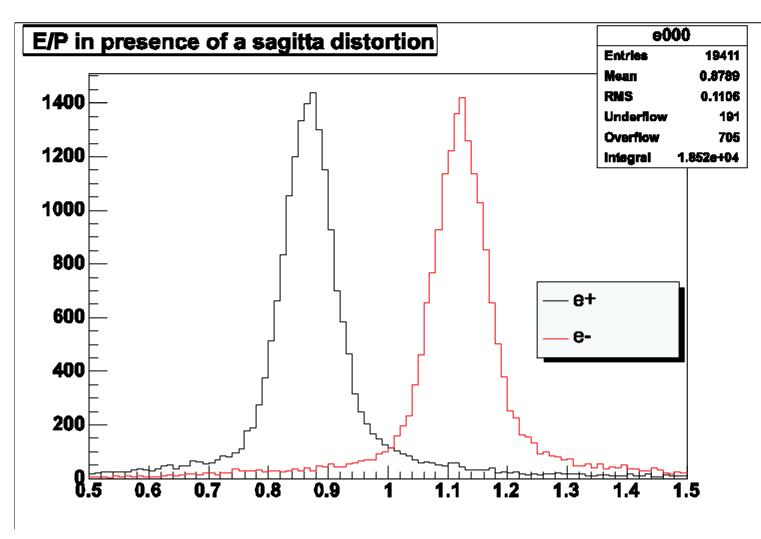
Plot E/p (E from calorimeter) for e+/e-Adjust detector until the two are the same Natural ~100 MeV e+/e- asymmetry in calorimeter (due to accordian structure?)
