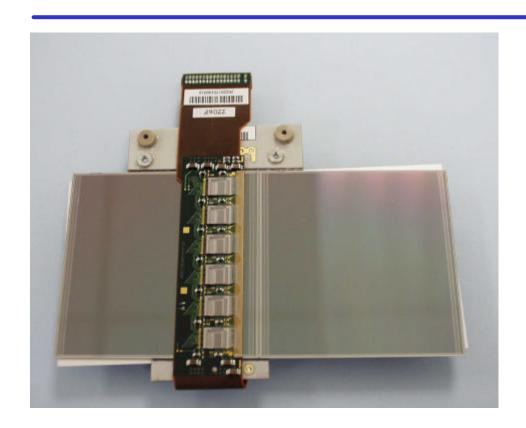
Focus on aligning the 7 barrels of silicon detectors
