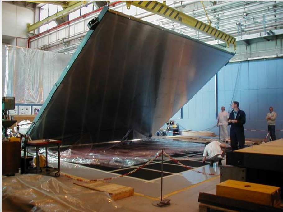
RICH2 exit and entrance windows
