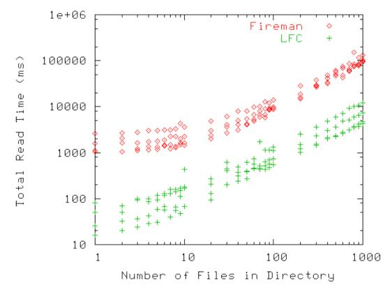
• Read performance measures the time the readDir operation takes for increasing number of files in the directory and threads. Results are shown for 1,2,5 and 10 threads with Total read time decreasing for increasing threads.
