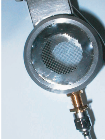
Figure A.5: 12.9 GHz cavity used by ASACUSA to measure the hyperfine structure of antiprotonic helium. It has an inner diameter of 28.8 mm, and uses meshes on both top and bottom of the cylinder to let antiprotons and laser beams pass. The microwave radiation is provided by a rectangular wave guide from top, and the magnetic field strength in the cavity is monitored by a pick-up antenna attached below.
