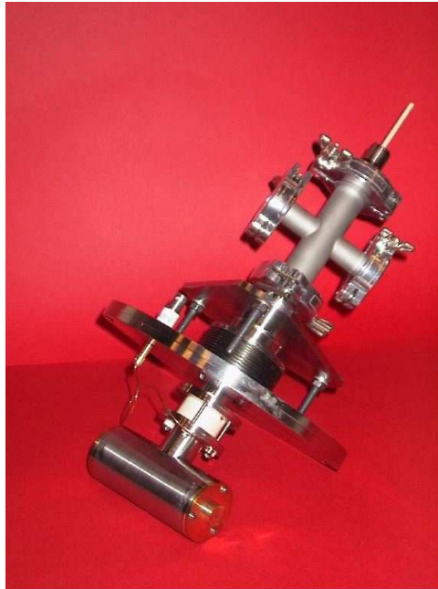
Figure E.5: The gas cell. It is mounted on an insulator, so that we can change the impact energy without retuning the ASACUSA RFQD, which facilitates the measurements at varying projectile energies.
