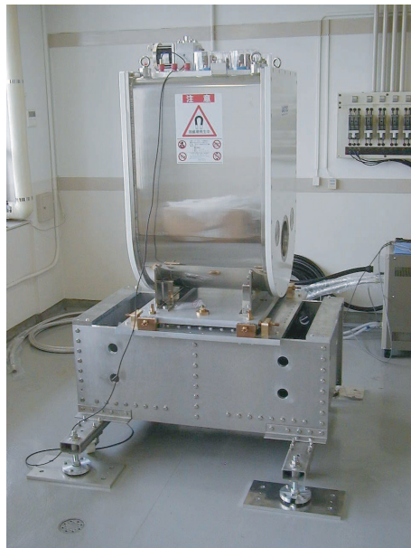
Figure C.8: Photograph of the superconducting quadrupole magnet.
