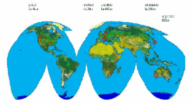
Many interferometric gravitational wave detectors across the world LIGO detectors (2x4km, 1x2km) in Livingston/Hanford USA GEO detector (600m) UK/Germany collaboration VIRGO detector (3km) France/Italy TAMA detector (300m) Japan
