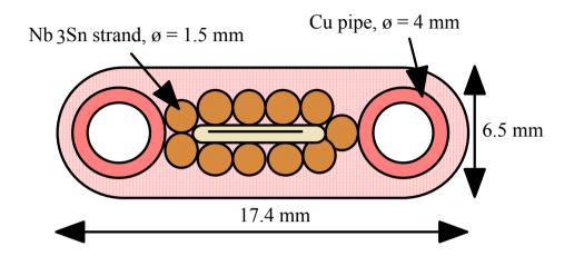
**Cooling:** forced flow, on two copper pipes, 4 mm inner diameter, hydraulic length  $\approx 200$ m **Supercondutor:** 11 multifilamentary, non-stabilized Nb<sub>3</sub>Sn strands cabled on a bronze strip **Assembly:** pipes and strands are bonded *after heat treatment* by electroplated Cu, 1.2 mm thick
