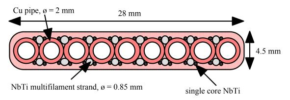
Cooling: forced flow, 2-phase He @ 4.5K in a linear array of nine copper pipes, 2 mm inner diameter, hydraulic length  $\approx 200 \text{m}$
