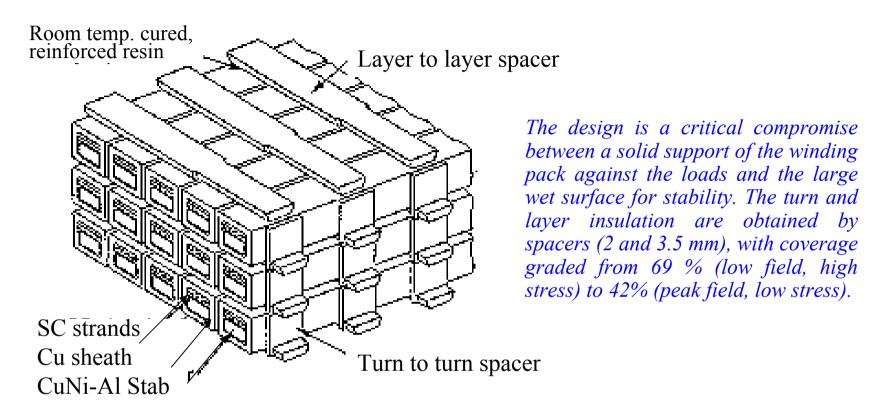
The expected cryo-stability, based on cold-end recovery, was actually not fully achieved. The operating current had to be limited to 11.3 kA due to observed propagating normal zone. Subcooled operation is planned at 3 K to improve stability
