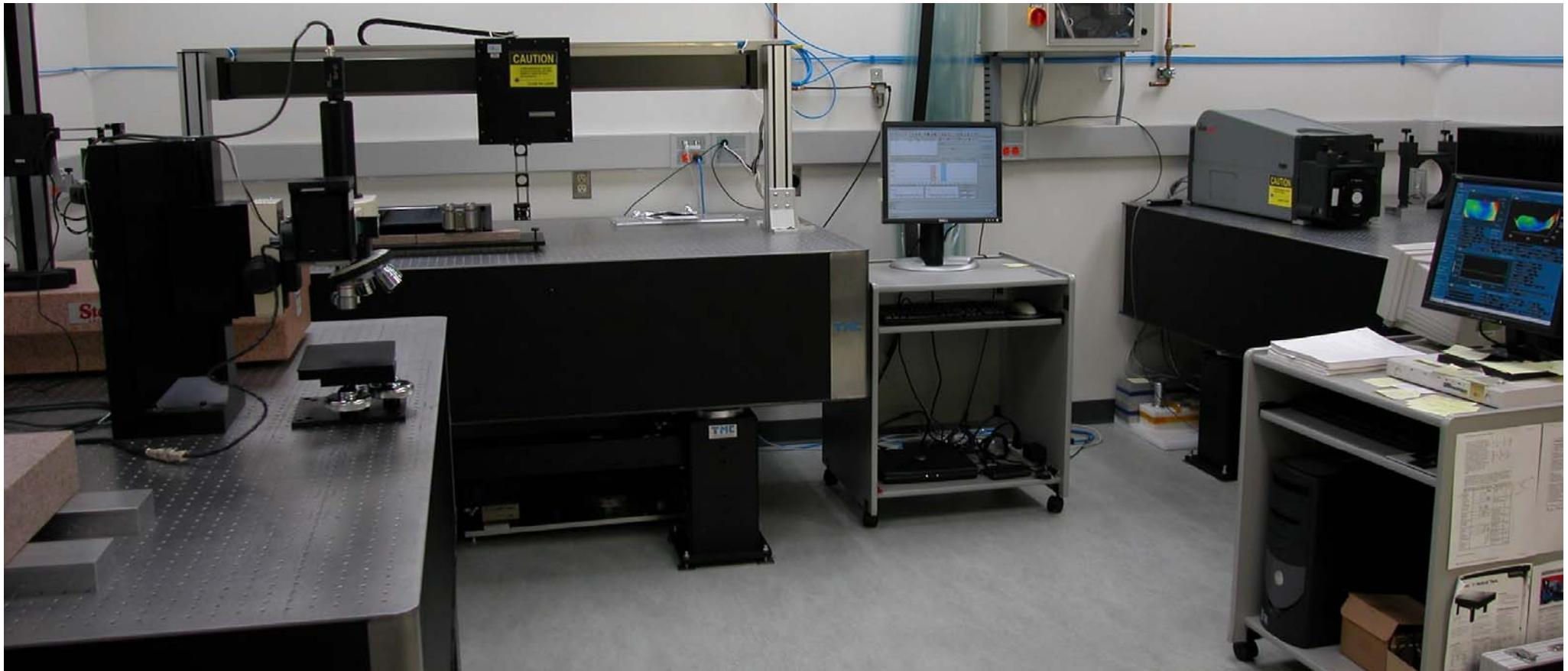
Purpose: To ensure quality of Synchrotron optics prior to their installation into a beamline. Radius of Curvature, Slope Error and Surface Roughness can be measured using the three main measurement instruments.
