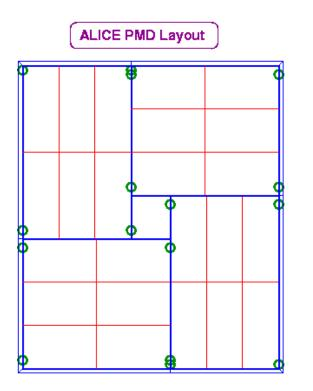
O ---- Positions of fiducial markers on the Supermodule boundary - 16 Nos/plane Two detector Planes: CPV and Preshower
