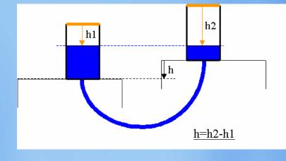
Continuous monitoring of the relative position performed by the sensor's surface (electrode) and the water surface (target). Capacitive measurements determine the distance to the target.
