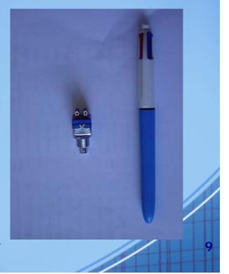
Switches on the normal magnets of the LHC (IR3 & IR7). (Thermoswitchs ELMWOOD 3106 – T117 - buttons SECME C4, connectors BURNDY 4BPM, Kapton cables)
